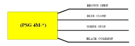
\* Home Automation System is to supply to EACH conductor a Momentary Dry Contact, Normally Open. (3-Contacts Total: Open, Close, & Stop)
